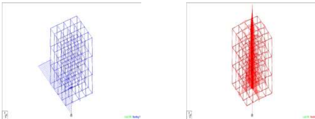
Figure 6. Analysis Of Irregular Structure Minor Axis And Major Axis Moment
